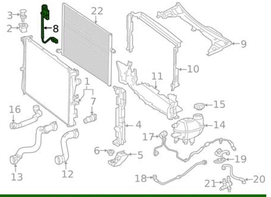
Part or sub-assembly is #8 in diagram Diagram may not be specific to your vehicle
