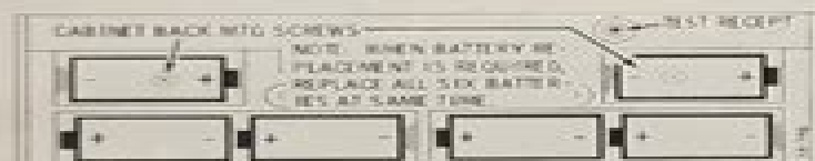
REAR VIEW OF RADIO WITH PANEL REMOVED SHOWING BATTERY LOCATIONS
