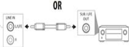
LFE OUTPUT - LFE Output on Processor/Pre-Amp/Receiver connected to LFE input on subwoofer amplifier
