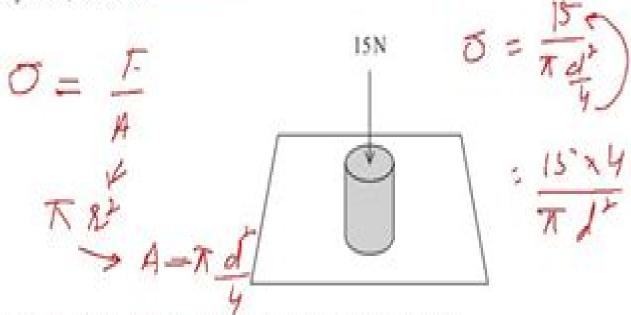
The stress in the cylinder, in pascals, can be calculated using
