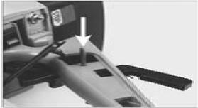
Dismantle the spring and throttle control lock.
