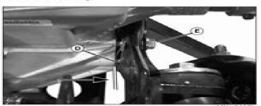
Carefully lower transmission into machine. Place new gasket on pins. Ensure that the gasket stays in place and the alignment pins (D) start to seat in right-hand bearing holder side plate.
