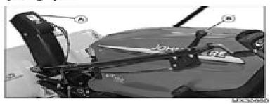
The distance snow will be discharged can be adjusted by moving snow deflector (A).
