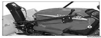
Turn chute control rod (A) to right to direct snow to right side of machine and to left for opposite effect.
