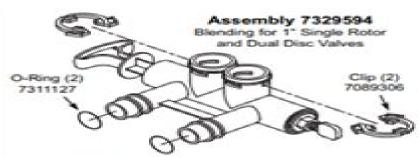
Parts: 7328530 Stem 7173016 O-Ring, Stem (4) 7175238 C-Ring 7307518 Blend Screw 7129635 Lock Nut 7329609 Clip, Blend Screw 7183590 O-Ring, Blend Screw (2)
