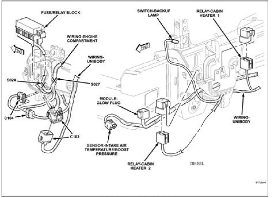
Fig. 12 FRAME RAIL - LEFT FRONT (DIESEL)
