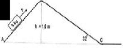
Calculate the magnitude of the force F if the power that is used to move the box the incline AB is equal to 57,6 W.
