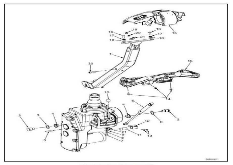
Figure 3. Control Handle Assembly
