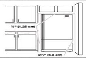
To ensure proper ventilation for your refrigerator, allow for a 10' (1.25 cm) space on each side and at the top. Allow for 1' (2.54 cm) of space behind the refrigerator. If your refrigerator has an ice maker, make sure you leave some extra space at the back for the water line commections.
