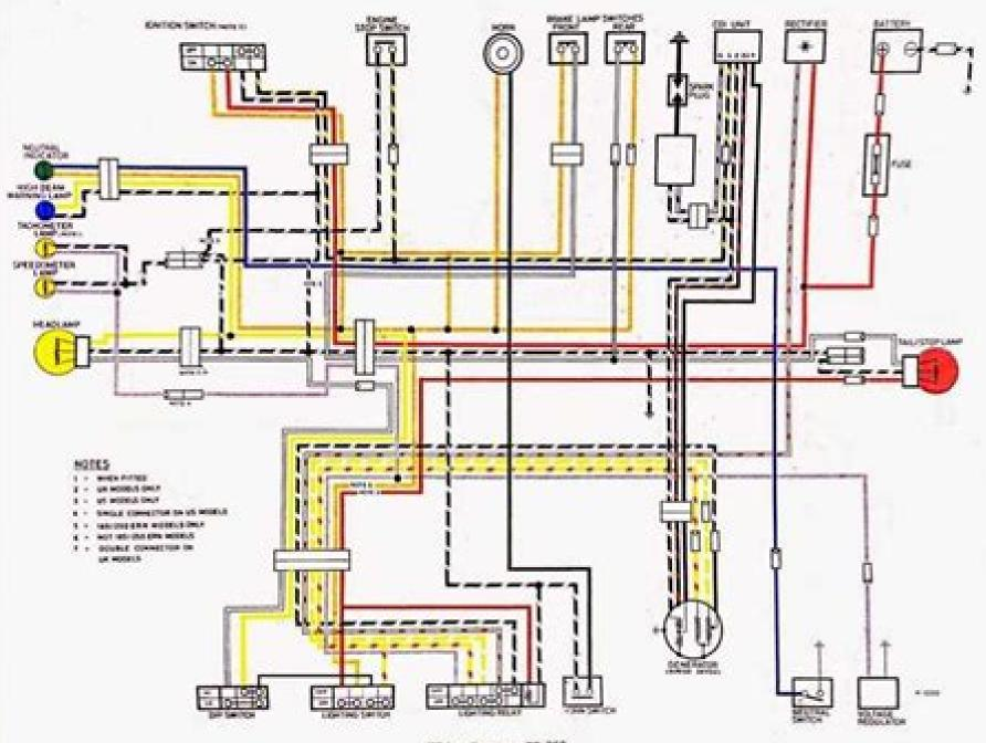
Wiring diagram - TS 250
