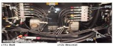
While moving the bracket, turn the DPF muffler vertically so it can be removed.
