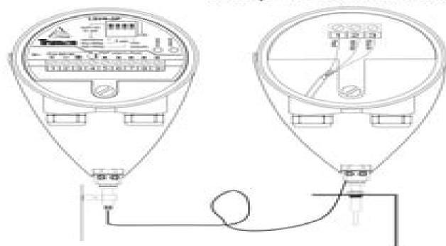
Proper connection to supply earth terminal (3) and the external earth terminal (screw) is must.
