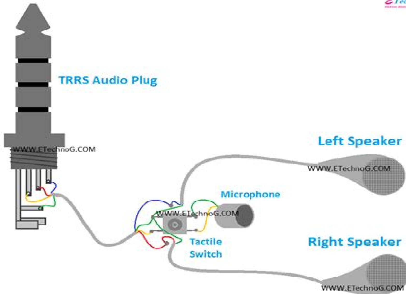
Stereo Headphone Jack Wiring and Connection Diagram
