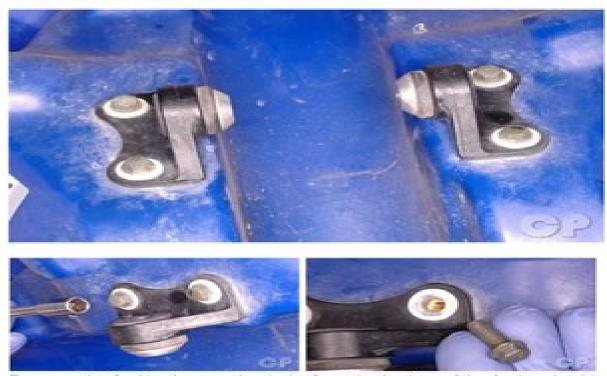
Remove the fuel tank mounting bolts from the bottom of the fuel tank with an 8 mm socket.
