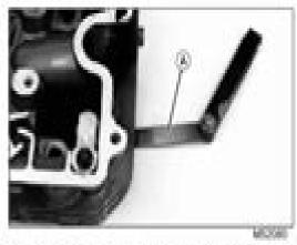
Put head on a flat surface plate. Check for distortion at several points with a feeler gauge (A). Replace head if distorted beyond specification.
