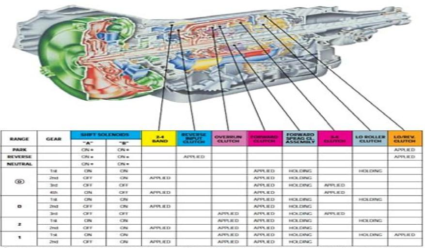
SOLENOID "A" & "B" OPERATION AND THE SHIFT VALVE POSITIONING IN P.R.N. RANGES ARE A FUNCTION OF THE INPUT TO THE SOLENOIDS FROM THE VSS. UNDER NORMAL OPERATING CONDITIONS THE SOLENOIDS ARE ON IN P.R.N.
