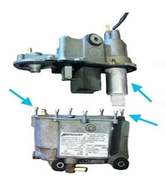
Mercury canister is disassembled by removing 7 screws, which reveals the fuel pump motor which slides out for easy removal and replacement
