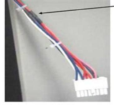
Check the splices for good connection integrity
