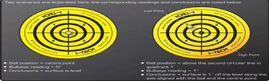
NOTE: For the purposes of this illustration a 350mm diameter subsea bullseye x 2° measurement scale has been used nominally. Other bullseye sizes and measurement scales will vary in appearance however the general principles apply across the range.
