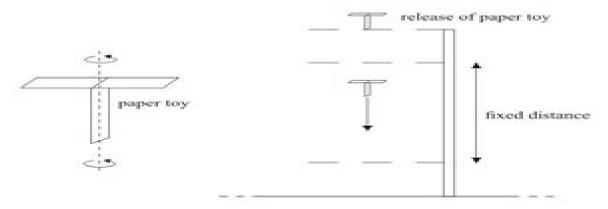
The aim of the experiment was to find how the terminal speed of the paper toy varies with its weight. The weight of the paper toy was changed by using different numbers of paper sheets in its construction.
