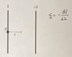
The distance x is measured from point P in the direction perpendicular to the plate.
