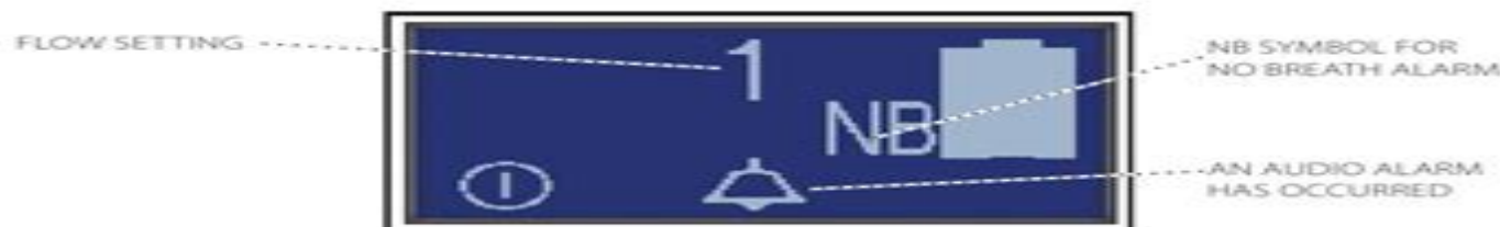
Figure 18. Example of an alarm screen. If the device does not detect breathing for 120 seconds, it will sound the NB alarm and show this typical display with the NB alarm symbol (NB = No Breath). The alarm symbol (bell) shows the audio alarm is on. To silence the audio alarm, press the alarm symbol. For a complete list of alarms, see the Alarm Indicators section of this manual.
