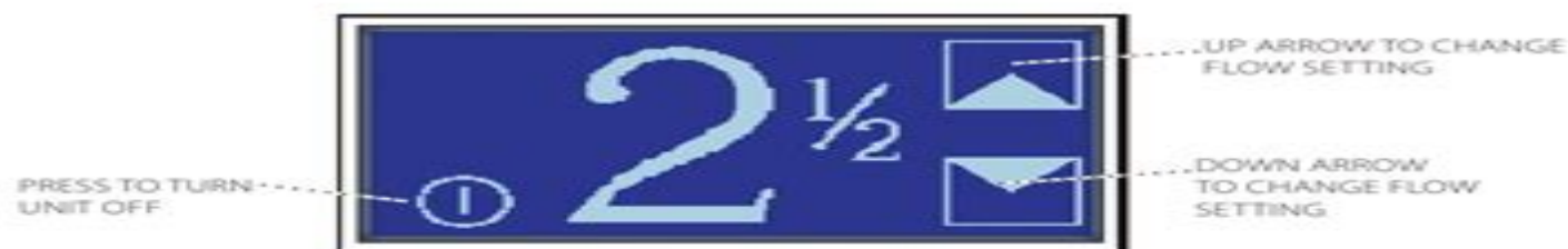
Figure 17. To change the flow setting, touch the setting number; here it is 2 1/2. This causes the up and down arrows to appear. To increase the flow setting, press the up arrow on the right until you reach your prescribed setting. To decrease your flow setting, press the down arrow. The flow setting arrows disappear when you touch the number again or 5 seconds after you last touched the screen.
