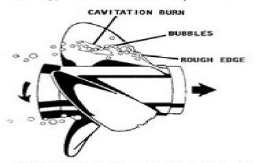
Constation (air bubbles) formed at the propeller. Manufacturers are constantly fighting this problem, as explained in the text.
