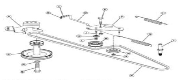
A - Belt GuideBelt guide removed at serial number 200000. Machines above serial number 200000 have built guide built into the engine mounting plate.
