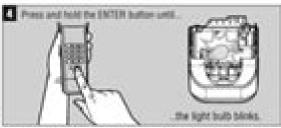
To test, press the PIN, then press the EATER button. The garage door opener will activate. To program the Keyless Entry to more than one garage door opener, repeat the steps above using a new PIN for each additional garage door opener.
