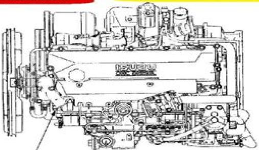
Engine coolant temp sensor
