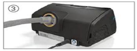
Connect the air tubing firmly to the air outlet located on the rear of the device.
