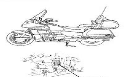
The engine serial number is stamped on the rear right side of the engine case.
