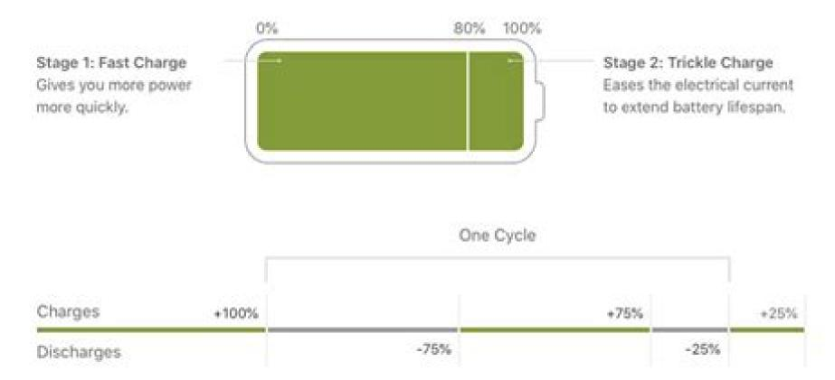
One charge cycle is completed after you've discharged 100 per cent of your battery's capacity.
