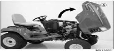
Lift rear of hood (A) and tilt to fully upright position.
