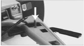
Dismantle the spring and throttle control lock.
