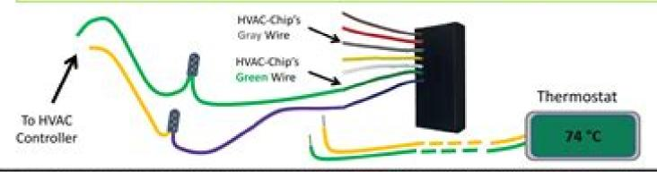
Basic Concept: Regardless of where at the Air Handler Unit the CWS-8THEM-0006 HVAC-Chip is installed, the GREEN and the PURPLE wires of this HVAC-Chip respectively always connect to the Fan and Compressor wires going to the HVAC system or HVAC controller. (See above picture)
