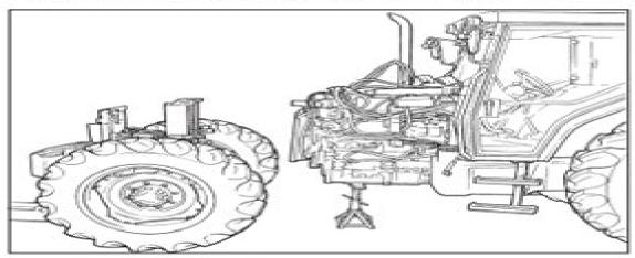
a) Position the tractor onto the rails and rolling stands, as shown in the illustration above.
