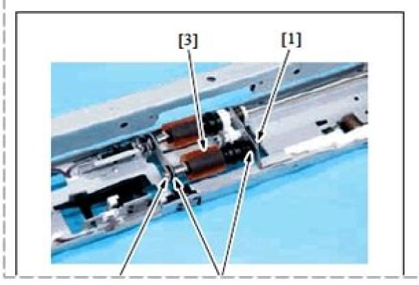
Remove two C-cli bearings [2], and feed tray 2 pick-up
