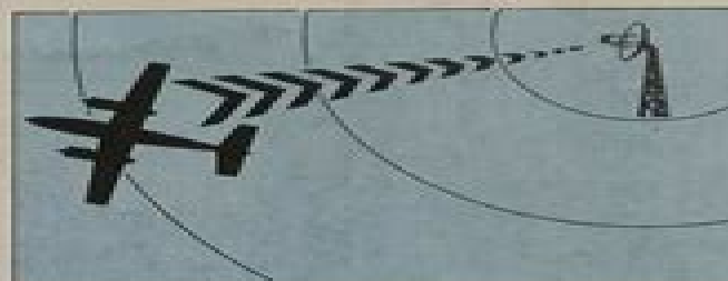
Transponder-pulsed transmitter replies to radar station.
