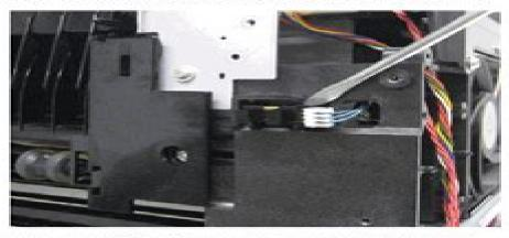
Note: It might take a small amount of force to remove the sensor (rear door interlock).
