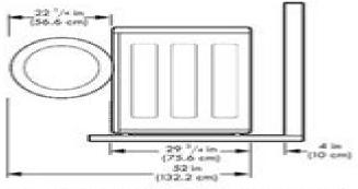
To ensure sufficient clearance for water lines and airflow, allow minimum clearances of at least 1 in. (2.5 cm) at the sides and 4 in. (10 cm) behind the unit. Be sure to allow for wall, door, or floor moldings that may increase the required clearances.
