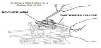
NOTE: Always check and adjust valve clearance while engine is cold
