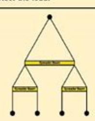
ONE OVER TWO INLINE SYSTEM Ideal solution for those lifts where long spans and potential bending of the load is a problem.
