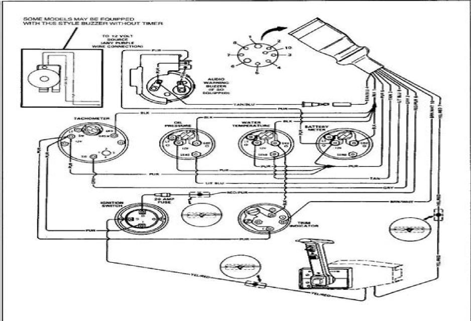
Fig. 174 Instrument harness wiring schematic—1992-97 V6/V8, single station (w/Quickstiver gauges)
