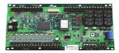
The LNL-1320 Dual Reader Interface (DRI) Module attaches to specific card reader devices. The interface is the communications link between the Intelligent System Controller (ISC) and the card reader.
