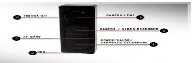
Note: Press 4,5 key to reset (when the machine encounter crash or not charging procedures disorder, please press two keys at the same time to reset)
