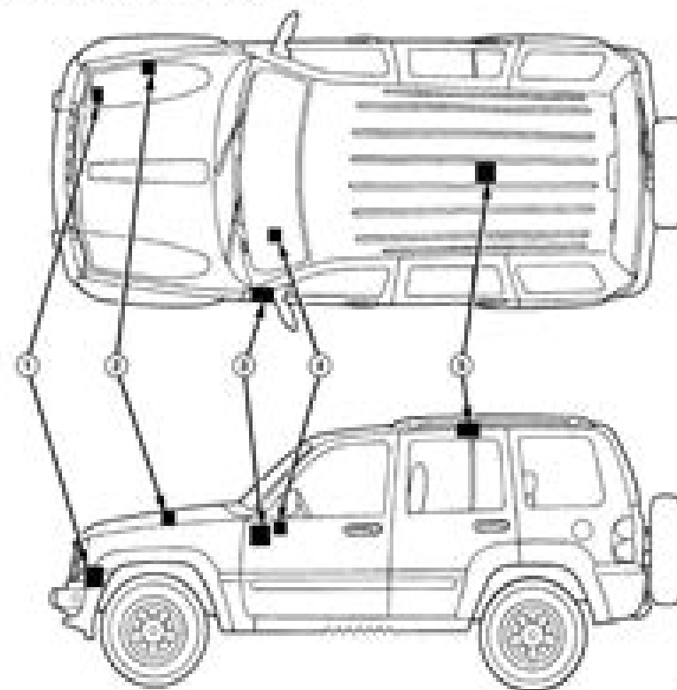
Fig. 1 Vehicle Theft Security System
