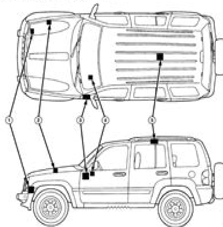
Fig. 2 Vehicle Theft Security System
