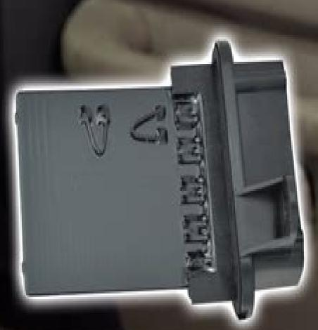
HOW TO REPLACE BLOWER MOTOR RESISTOR 1997-2006 JEEP WRANGLER
