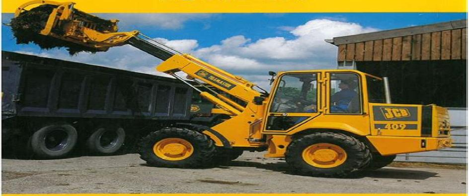
Lifts 2 tonnes to 4.3 metres • Places 1 tonne loads to forward reach of 3.4 metres
