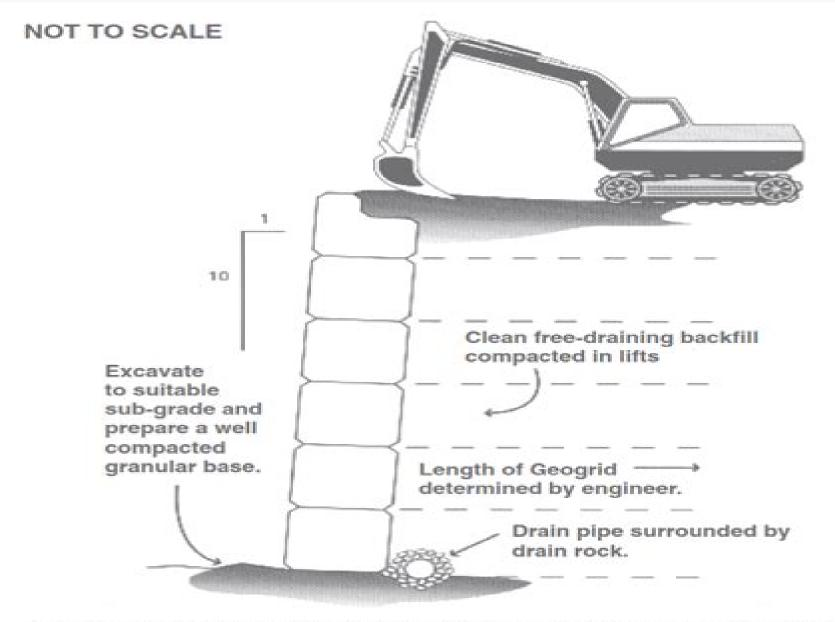
A vertical or near vertical wall is possible if a soil reinforcing geogrid is added to the backfill at every row of blocks. Very high loads can be supported with this type of construction. Ask manufacturer how to minimize geogrid wrinkling behind wall.
